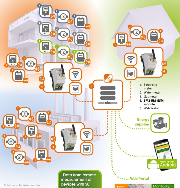
reading of electrometers, water meters, gas meters and connecting other devices, where we need to read pulses or binary status. The Solar Monitor modules together with the web portal make remote measurement and monitoring very easy and comprehensible.
