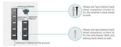
Warning: Before drilling, make sure to avoid the buried water tube and electric wires in the wall to avoid danger.
