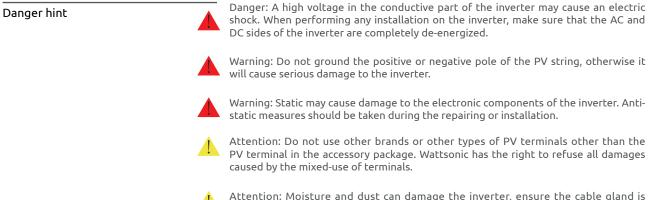
Attention: Moisture and dust can damage the inverter, ensure the cable gland is securely tightened during installation. The warranty claim will be invalided if the inverter damaged by the cable connector not well installed.
