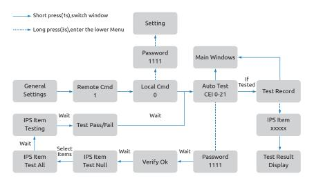
The auto test will start when the correct test item is selected, and the test result will be displayed on the screen when it finished. If the test success, it will display "Test Pass", otherwise will display "Test Fail". After each item tested, the inverter will reconnect to the grid and automatically start the next test item according to the requirements of CEI 0-21.
