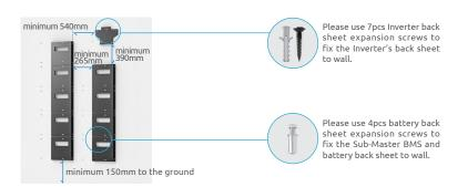
Warning: Before drilling, make sure to avoid the buried water tube and electric wires in the wall to avoid danger.
