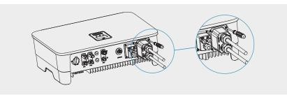
6) Lock the AC connector cover to the inverter with screws.
