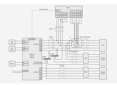
This diagram is an example for Australia and New Zealand. Neutral line of AC supply must not be isolated or switched.
