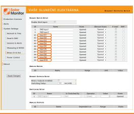
Checkbox shown below is used to select events in which an SMS is sent (e.g. the value from the sensor is outside the allowable range).
