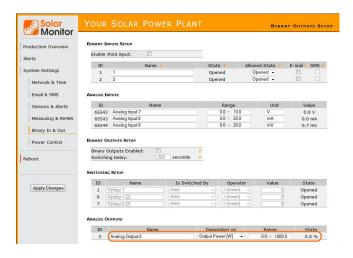
To correctly set the analog inputs a configuration list is needed. According to the configuration list, we discover the extent to which each input measure ((e. g. 0 - 20 mV). This range can be simply converted e. g. for measuring wind speed. If we know 0 m/s = 0 mV and 30 m/s = 15 mV then these values should be transferred to the measuring range:
