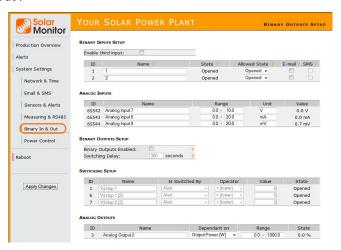
The settings of the digital outputs are the same as the output DO1 of SM2 - MU. The outputs must be enabled. Then select under what conditions, the outputs are switched (e.g. from a power value).
