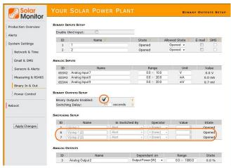
Analog output in a similar way as for the digital. We choose depending on what the output will be set (e.g. a room temperature with inverters). For this example we set a temperature range for the output value 0 - 10 V, which will regulate the speed ventilation.
